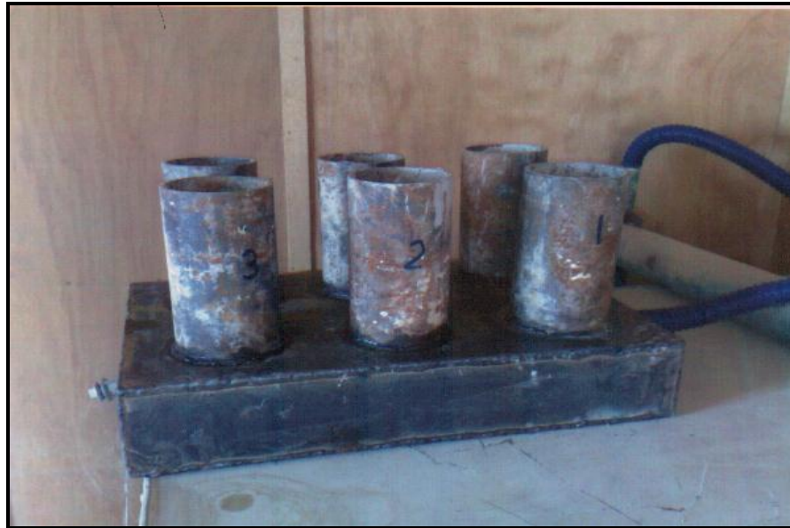
Figure (1): Lab apparatus used for treated sludge drying
